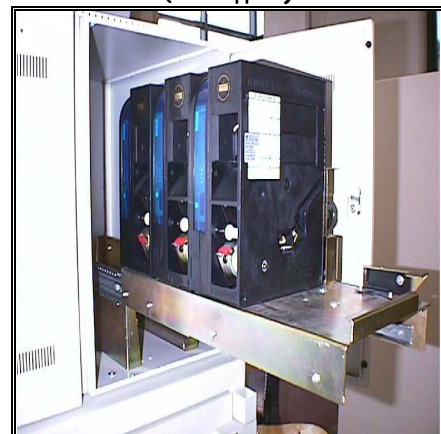
Internal view SAT300V (coin hoppers)
