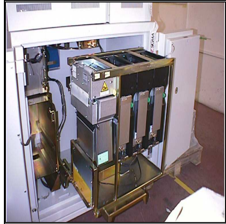
Internal view of SAT300V (banknote acceptor,final cash box,banknote dispenser)
