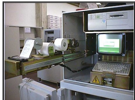
Internal view of SAT300V (ticket printer, Log printer with rewinder,PC,9"service monitor,key board for service personnel,UPS)
